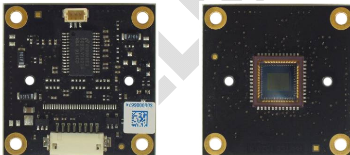
Figure 71: phyCAM-S (VM-009-LVDS) (rear / front view)
