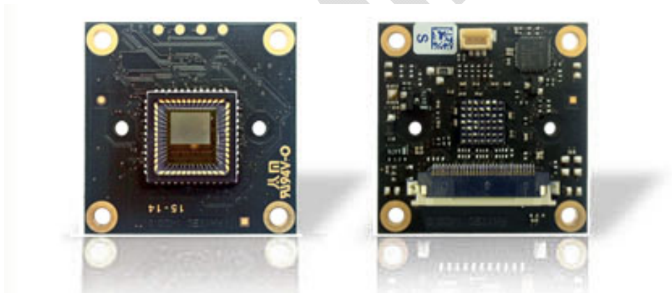
Figure 56: VM-012 (phyCAM-P) (front / rear view)
