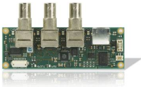
Figure34: Analog Video Digitizer (VM-008, PCB revision: PL1353.1)
