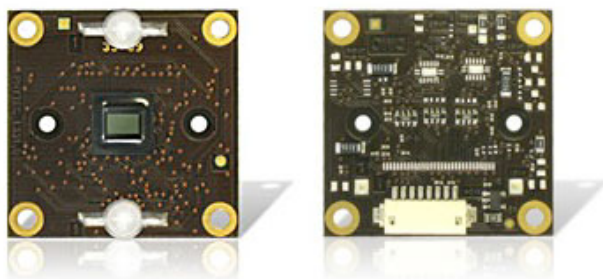
Figure67: phyCAM-S (VM-007-LVDS) (with LED-light, front- / rear view)
