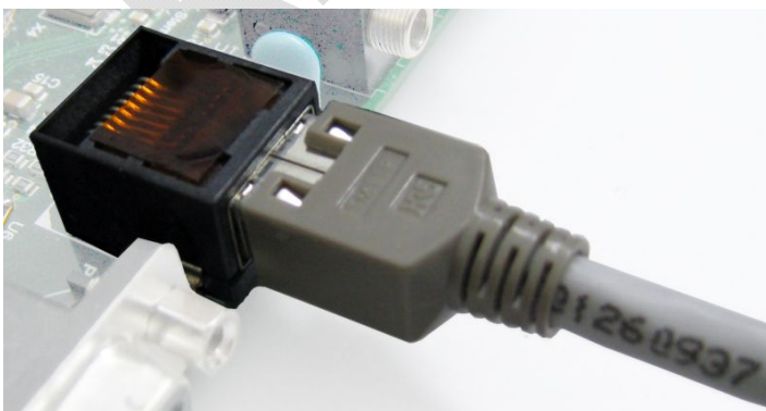
Figure14: RJ-45 Camera connection (phyCAM-S)
