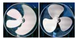
Rolling / Global Shutter: Shot of a rotating fan with different shutter technology.
