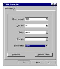
• Selecting *OK* advances you to the "COM1 Direct – HyperTerminal" monitoring window. Notice the connection status report in the bottom lower corner of the window.
