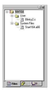
At this point you have created a project called *blinky2.uv2* and added an existing C source file called *blinky2.c* and an existing assembler file called *start164.a66*. Next you modify the C source before building your project. This includes compiling, linking, locating and creating the hexfile.
