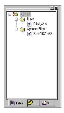
At this point you have created a project called *blinky2.uv2* and added an existing C source file called *blinky2.c* and an existing Assembler file called *start167.a66*. The next step is to modify the C source before building your project. This includes compiling, linking, locating and creating the hexfile.
