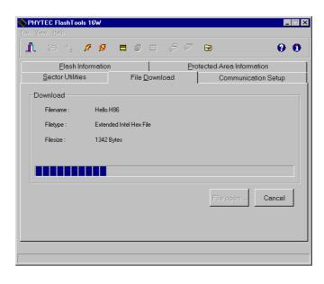
• At the end of the download, a sector by sector status check of the Flash-Memory can be viewed in the left-hand corner of the FlashTools 16W Worksheet window. Wait until the status check finishes before returning to work with the board. Once the status check is complete, the downloaded code can be executed.
