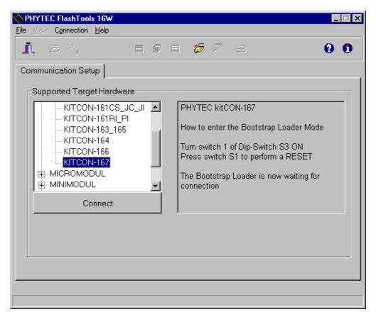
• Select the correct module from the list and press the *Connect* button.
