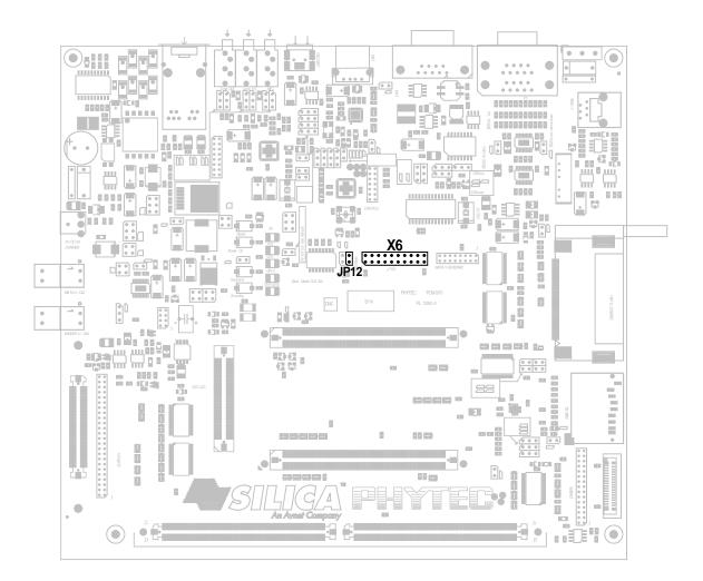
Figure 28: phyCORE-iMX Carrier Board JTAG Interface
