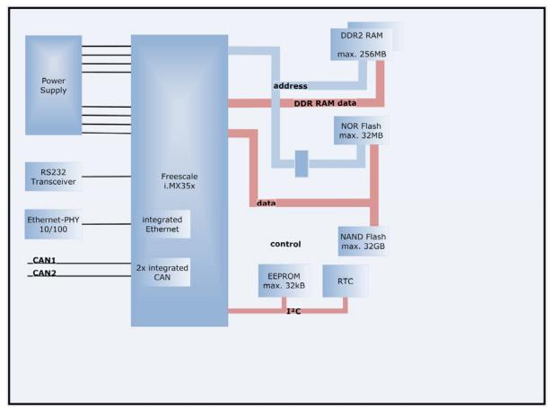
Figure 1: Block Diagram of the phyCORE-i.MX35
