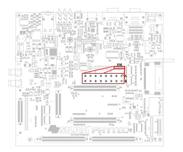
Figure 22: phyCORE-i.MX Carrier Board Keypad Interface
