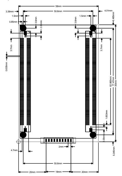
Figure 10: Physical dimensions of phyCORE-i.MX35 module
