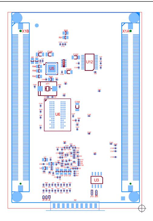
*Figure 3: Bottom view of the phyCORE-i.MX35 (connector si*de)
