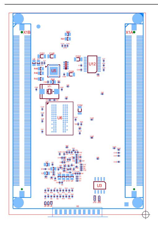
Figure 30: phyCORE-i.MX35 component placement (bottom view)
