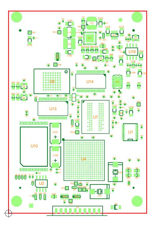
Figure 2: Top view of the phyCORE-i.MX35 (controller side)
