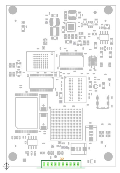
Figure 8: JTAG interface at X2 (top view)
