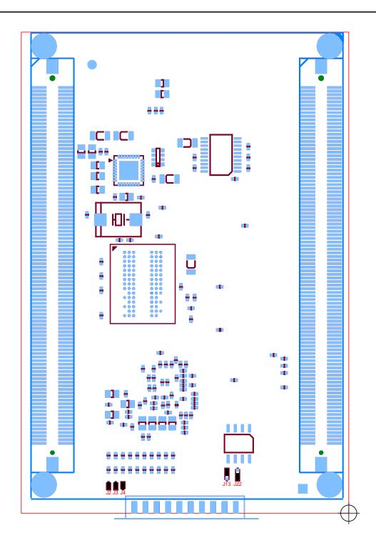
Figure 7: Jumper locations (bottom view)
