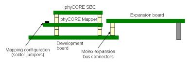
Figure 11: phyCORE-i.MX35 Carrier Board connection using the phyMAP-i.MX35
