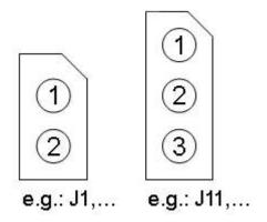
Figure 5: Typical jumper pad numbering scheme
