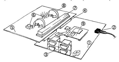
Figure 11: Modular Development and Expansion Board Concept with the phyCORE-XE167
