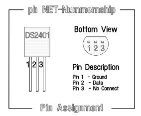
Figure 34: Pin Assignment of the DS2401 Silicon Serial Number
