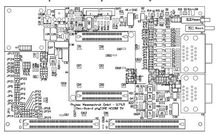
Figure 12: Location of Connectors on the phyCORE Development Board HD200 V3
