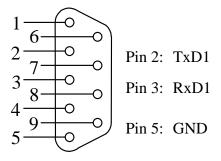
Figure 19: Pin Assignment of the DB-9 Socket P1B as Second RS-232 (Front View)
