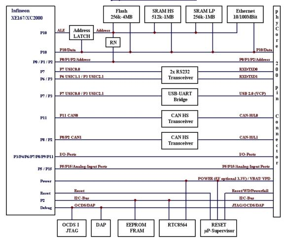
Figure 1: Block Diagram phyCORE-XE167
