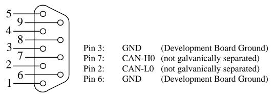
Figure 20: Pin Assignment of the DB-9 Plug P2A (CAN Transceiver on phyCORE-XE167, Front View)
