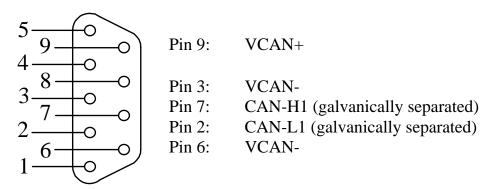
Figure 25: Pin Assignment of the DB-9 Plug P2B (CAN Transceiver on Development Board with Galvanic Separation)
