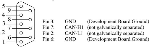
Figure 24: Pin Assignment of the DB-9 Plug P2B (CAN Transceiver on phyCORE-XE167)
