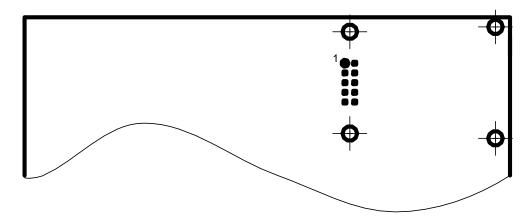
Figure 36: Ethernet Transformer Module Connector
