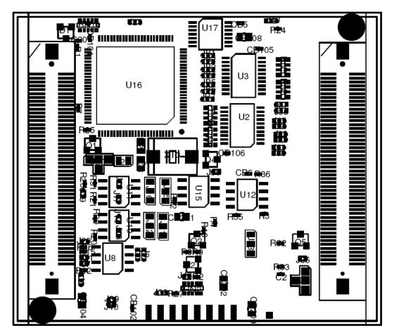
Figure 3: View of the phyCORE-XE167 (Bottom View)
