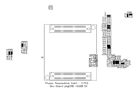
Figure 15: Default Jumper Settings of the phyCORE Development Board HD200 V3 with phyCORE-XE167
