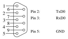
Figure 17: Pin Assignment of the DB-9 Socket P1A as First RS-232 (Front View)
