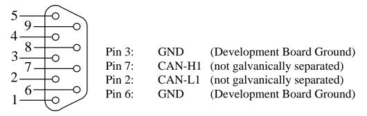
Figure 23: Pin Assignment of the DB-9 Plug P2B (CAN Transceiver on phyCORE-XE167)
