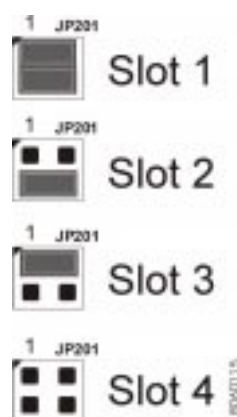
Figure 17: Jumper Settings JP201 (Slot Selection)
