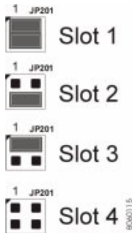
Figure 16: Jumper Settings of the Device-Selector JP201
