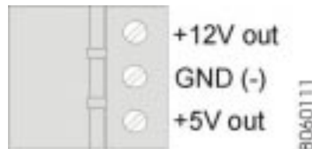
Figure 12: Connecting the Supply Voltage Output X302
