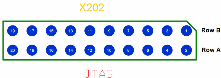
Figure 18: Development Board JTAG Connector X202
