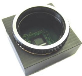
-H = camera with lens holder for C/CS-mount lenses
