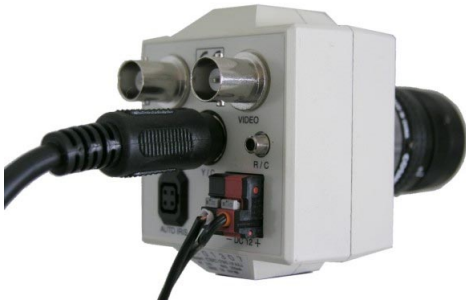
Figure 7: Camera Connector S-Video and Power Supply
