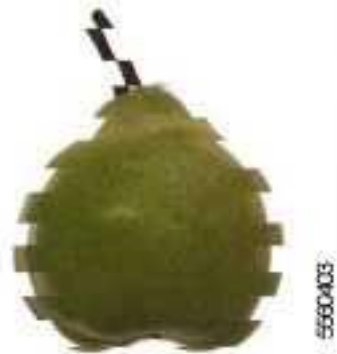
Figure 35: Comb Effect With Moving Objects in Frame Mode (Schematically)
