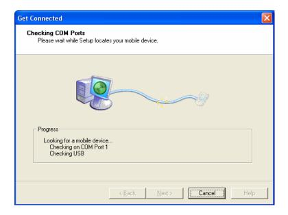
While Active Sync is looking for a connection click *OK* in the *Run*.. dialog on your PXA270 device to enable the connection to your device. Establishing the connection might take a few seconds. Once
