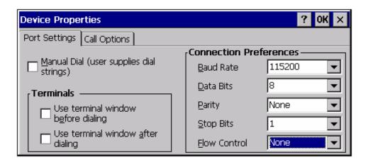
Leave all settings at default except for *Baud Rate* and *Flow Control*. Set the Baud Rate to 115200 and the Flow Control to *None*. Click on *OK* in the upper right corner. This will close the *Device Properties* dialog and you will return to the *Device* dialog. Click on *Finish* to create your new network connection. Close the network connection window.
