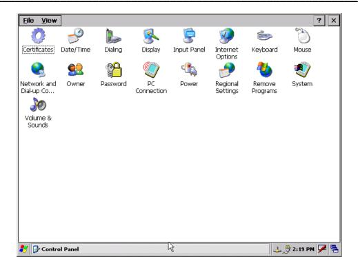
Double-click on the *Network and Dial-up Connections* icon. This will open a window that shows your existing network connections. Double-click on the *Make New Connection* icon.
