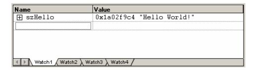
• The constant is shown with its address and a small sign in front which indicates that **szHello** is an array with a group of array elements. Click the sign to expand the view and to see all array elements of **szHello**.
