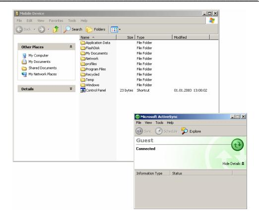
Open a file manager and navigate to the WinCE-Xscale-Disc in your CD-Rom drive. Go to the *WinCE50/Demo* folder. Select HelloWorld.exe and copy it to the *Mobile Device* window in the folder *FlashDisk* using drag and drop.
