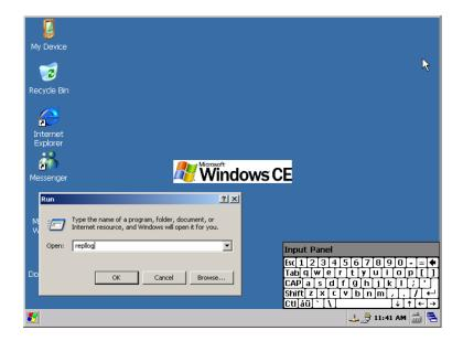
The program *repllog* will enable your device to connect with Active Sync which is running on your PC. Do NOT press *OK* yet. Instead click *Next* on the *Get connected* dialog running on your PC. This will cause Active Sync to start looking for a connection to a mobile device.
