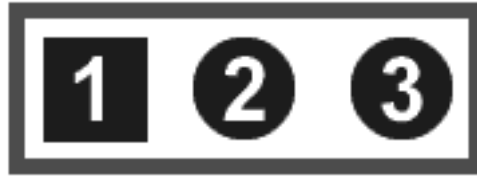
Fig. 19-2. Typical Jumper Pad Numbering Scheme (Removable Jumpers)
